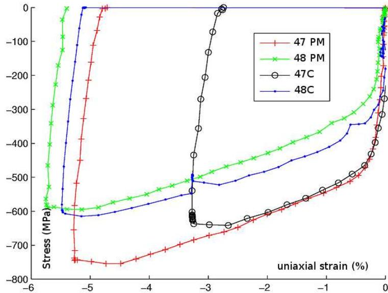
Figure 4: Macroscopic responses of the four specimens for uniaxial compressive tests.
