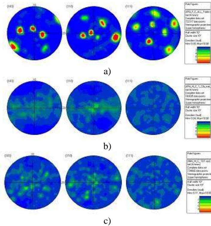
Figure 3: Crystallographic texture associated with orientation imaging microscopy. a) fully lamellar microstructure of 47C, b) near  $\gamma$  microstructure of 47PM, c) near  $\gamma$  microstructure of 48PM. Each analysed surface area is  $1 \text{ mm}^2$ .
