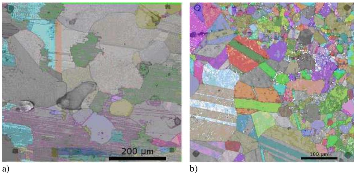
Figure 2: Orientation imaging microscopy of Ti-Al<sub>48</sub>Cr<sub>2</sub>Nb<sub>2</sub>. a) casting route b) powder metallurgy route.
