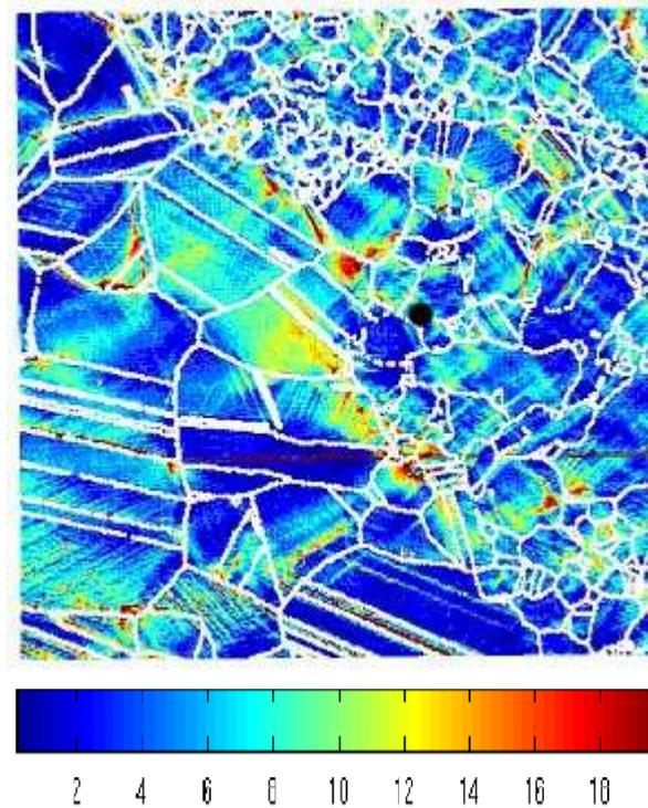
Figure 5: Superimposition of the Von Mises equivalent strain field with the microstructure for the 48PM material, for a macroscopic strain (vertical axis) of  $-5.5\%$  and a gauge length of  $2\ \mu\text{m}$ . The colour scale represents the magnitude of the strain [%].
