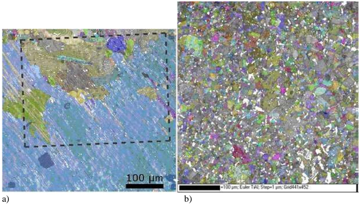
Figure 1: Orientation imaging microscopy of Ti-Al<sub>47</sub>Cr<sub>2</sub>Nb<sub>2</sub>. a) casting route. The dashed line represents the contour of the DIC imaging analysis area. b) powder metallurgy route.
